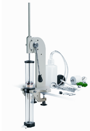
Figure AA3 Filta-Max® manual wash station (with assembled tube set and filter in place)
