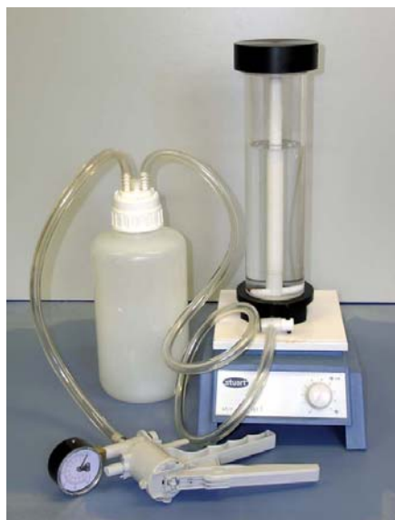
Figure AA5 Filta-Max® concentration tube set with stirrer assembly, on a magnetic stirrer and connected to a catch-bottle and vacuum pump
